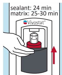
3. Close shield, press button and processing starts
