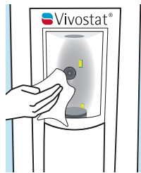
9. Clean centrifuge area with soft pre-moistened cloth, allow to dry
