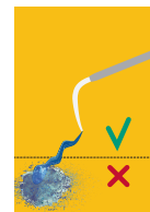
5. Verify correct mix on pH-paper (from liquid to viscous in 10-30 sec.)*
