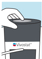
1. Press button to start loading syringes
