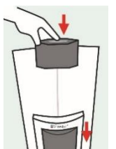
1. Press button to open shield
