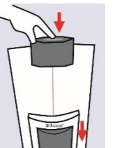
1. Press button to open shield
