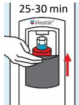
3. Close shield, press button and processing starts
